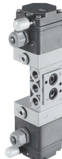
Fig. 3: 5/2-way solenoid valve · Actuated on both sides · With two detent positions · K_{VS} 1.4 · G \frac{1}{4} connection, NAMUR
