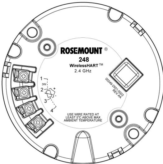
Figure 2. 248 Wireless Sensor Connection
